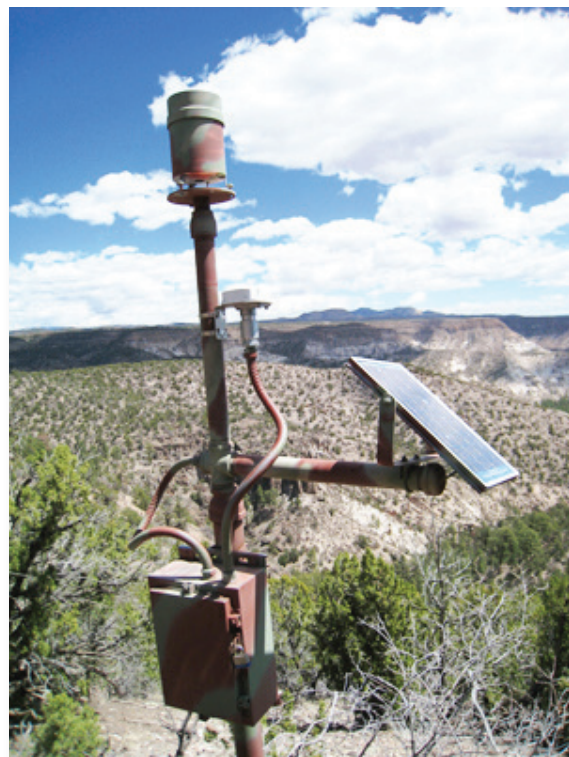
OneRain's StormLink® Satellite Telemetry installed in the Cochiti fire burn area in northern New Mexico. Real-time data are transmitted to OneRain's secure data storage center for web-based viewing, and 24/7 monitoring via Contrail®
